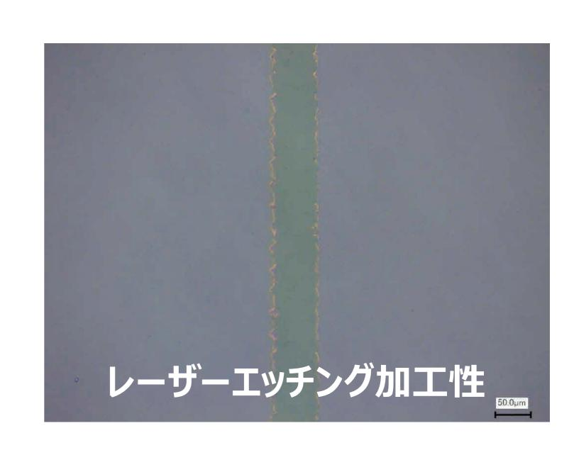
下地の隆起や透明導電膜のバリが少ない It has less bulges on the base and fewer burrs on the transparent conductive film.
